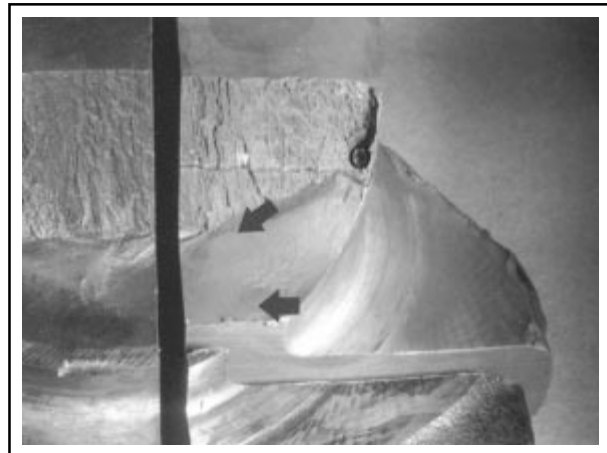
Fig. 10 Diagonal/circumferential fatigue fracture adjacent to the woody textured fracture
