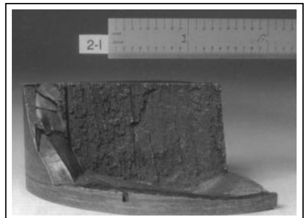
Fig. 7 Woody textured fracture on Crank #2, pin #2
