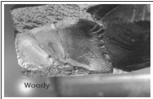
Fig. 9 Fatigue crack progression outwards from the woody texture of fracture towards the journal surface
