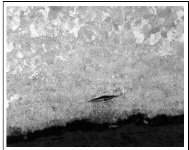
Fig. 14 A band of martensite found at the woody textured fracture edge
