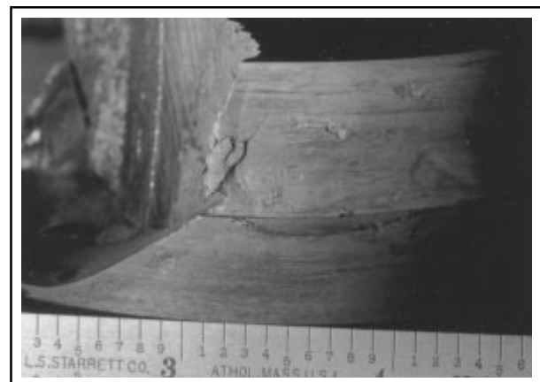
Fig. 3 Severe wear and spalling near the center journal surface on Crank #1
