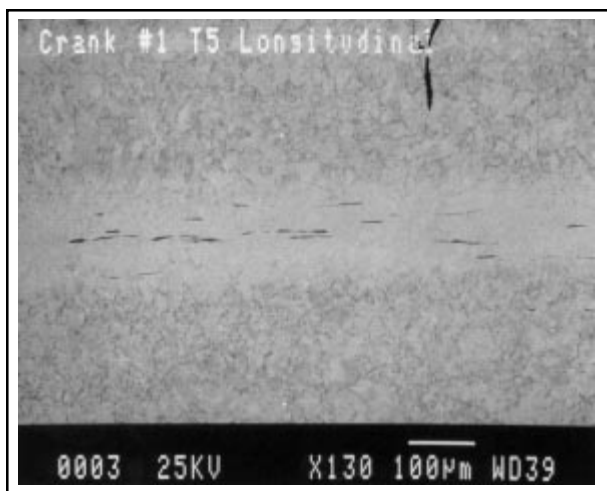
Fig. 21 SEM backscatter electron image of MnS inclusions surrounded by tempered martensite in Crank #1, pin #5
